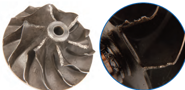
Damage to inducer of turbine wheel
